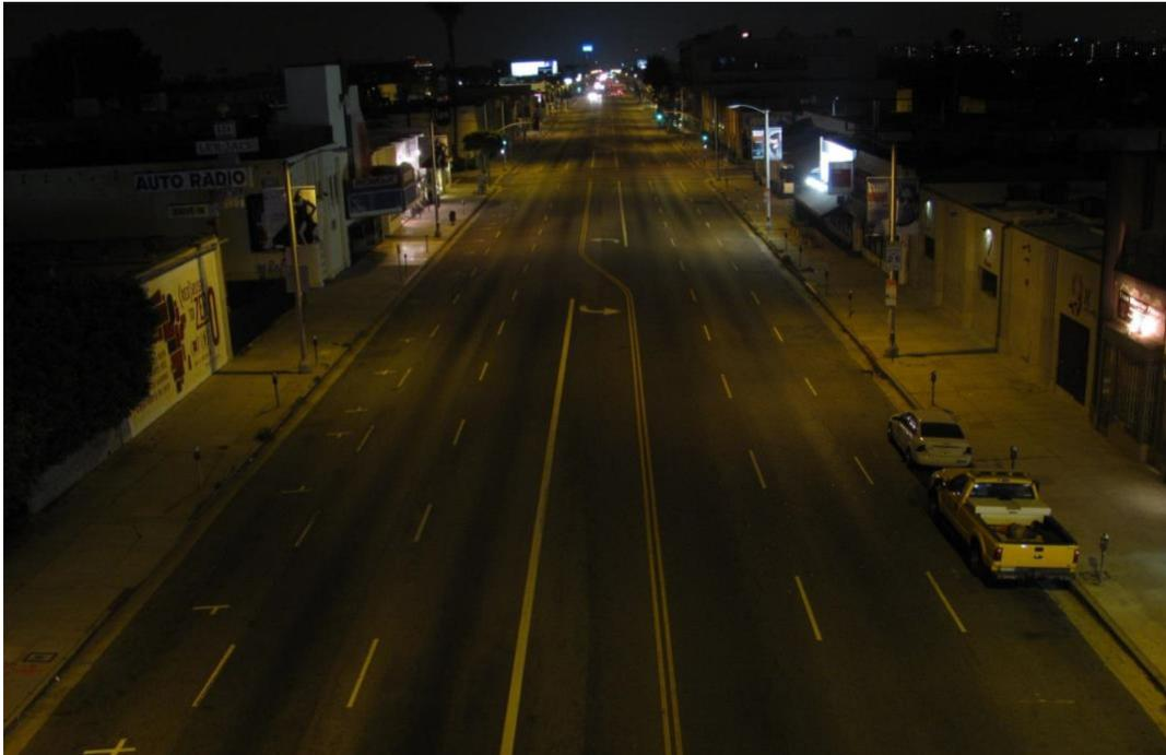
Figure 1 - A Los Angeles street illuminated by 200w HPS, just prior to LED conversion.
